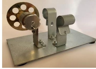
Fig.5. Stirling Engine base and piston
