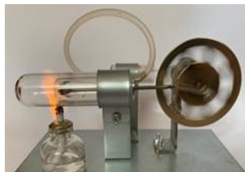
Fig.7. The two-piston Stirling engine
